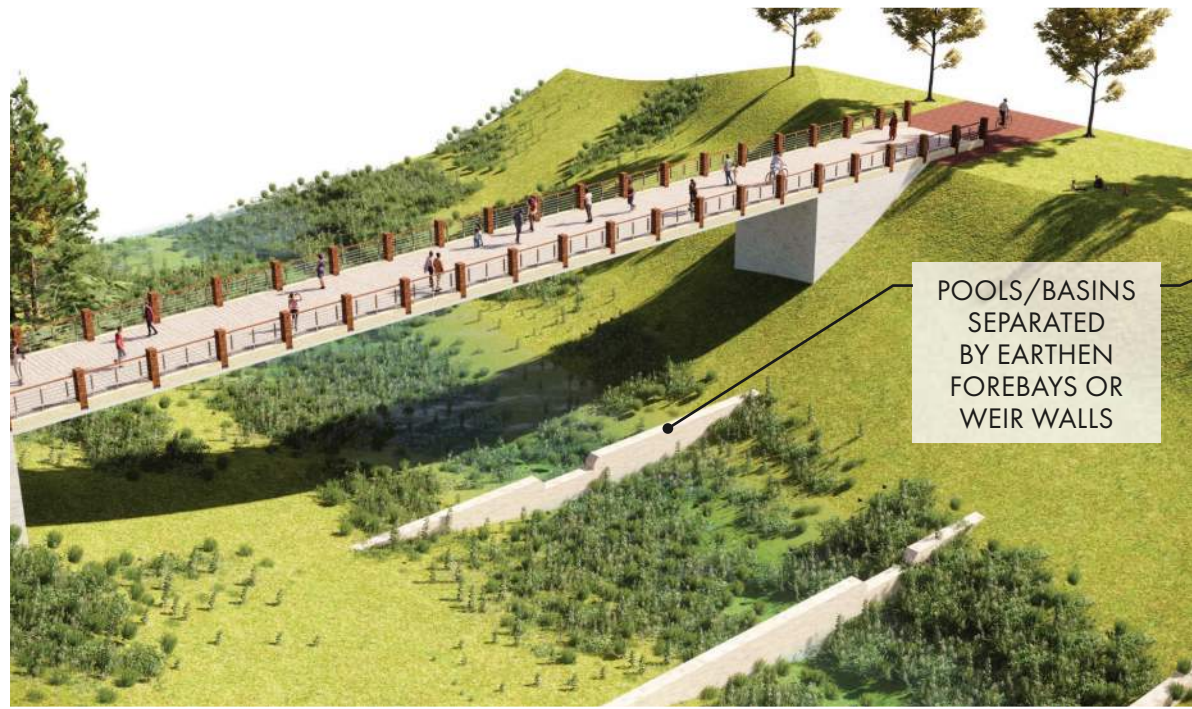
Vignette of Stormwater Chain pools/basins with weir walls under the Ravine Bridge
